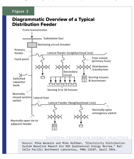
Finally, electricity is delivered to end users, either individuals or groups, again after transformers lower the final voltage.
